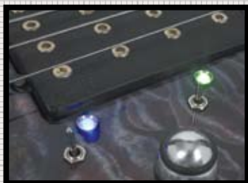
■ The colour of the high-brightness LEDs indicates what mode the pickup is in
